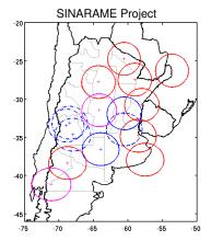
FIGURE – Weather radar network nowadays (blue line) and SINARAME radars (red line). Simple-pol (dash line) and dual-pol (solid line) radars.
