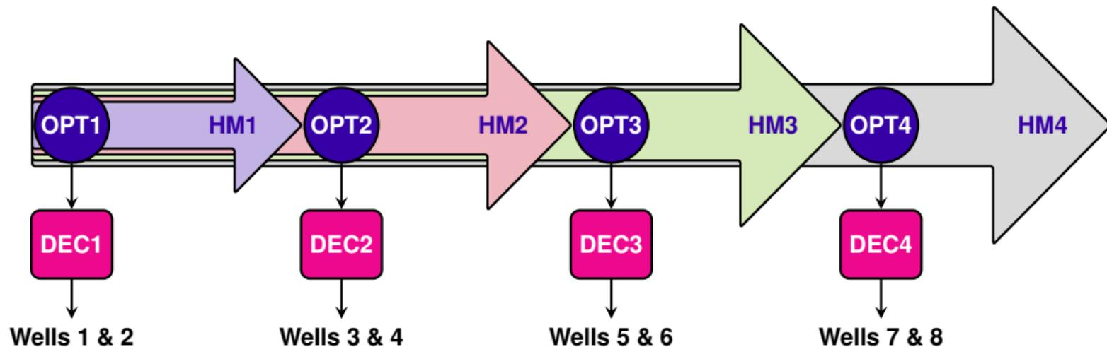
DIGIRES decision workflow for field development. Drilling two wells per year, we use the workflow to decide on the optimal drilling schedule.
