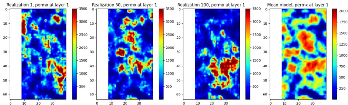
Permeability of Layer 1 on selected geological realizations and the mean model.
