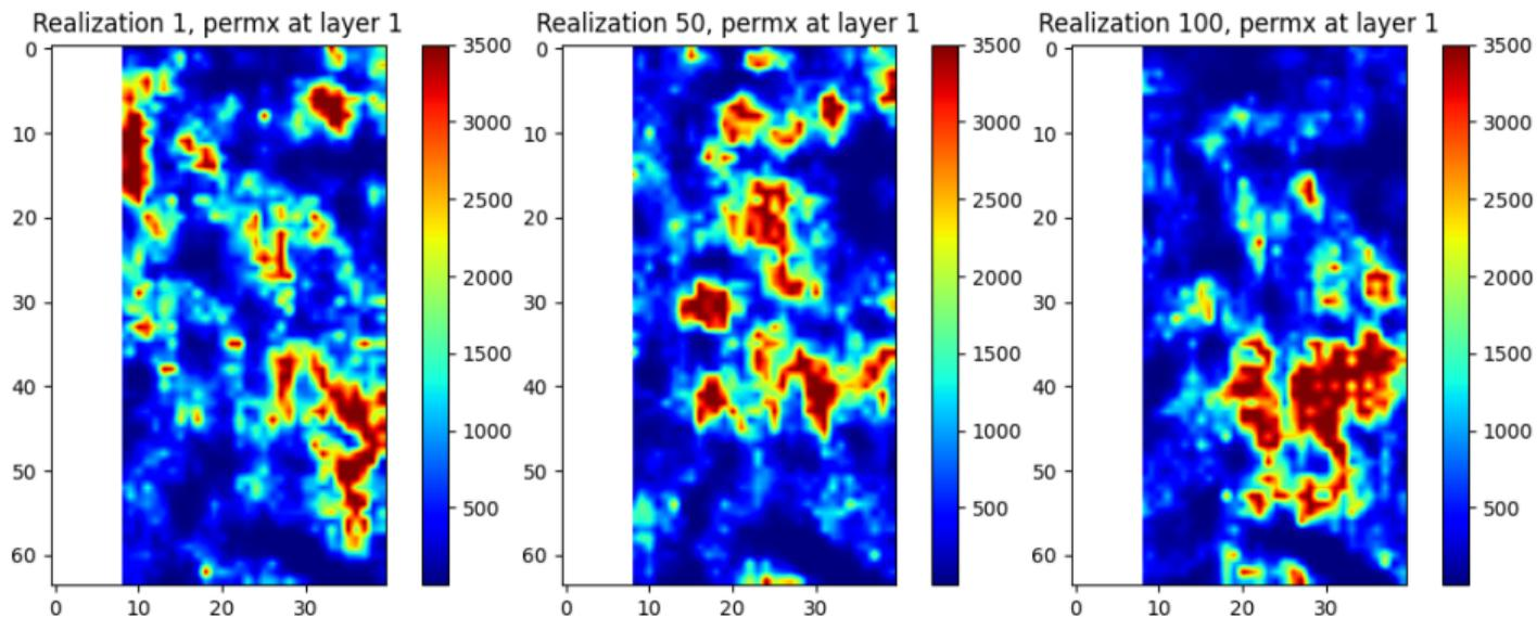
Permeability of Layer 1 on selected geological realizations and the mean model.
