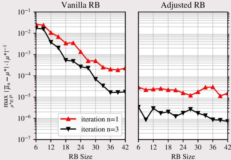
when the measurements bias is not corrected, the relative error is strictly dependent on the RB model accuracy
