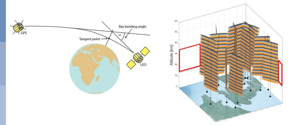
Temperature profiles are very accurate in the stratosphere (between 10-50 km). They are good for highlighting errors/biases
