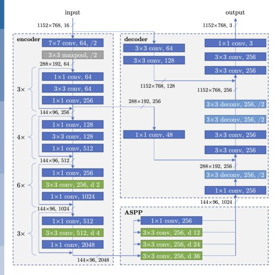
Convolutional neural network (CNN) are the best to learn computer-vision task. The usual 3 channels (RGB) have been replaced by 45 channels (vertical levels in the stratosphere)
