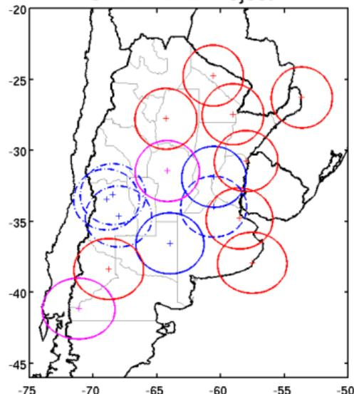
FIGURE – Weather radar network nowadays (blue line) and SINARAME radars (red line). Simple-pol (dash line) and dual-pol (solid line) radars.
