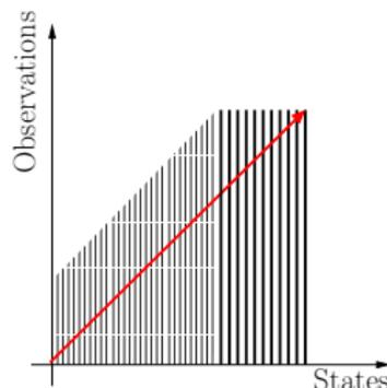
$$p(x_{t-L:t} | y_{1:t}) = p(y_t | x_t) \int p(x_t | x_{t-1}) p(x_{t-1-L:t-1} | y_{1:t-1}) dx_{t-1}$$
